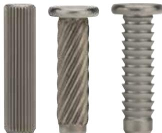
Barbs are recommended for use in flexible plastics where optimum resistance to axial force is desired. After installation, the plastic will backfill into the area around the barbs resulting in maximum retention. Barbs are not appropriate for brittle plastics or those containing high percentages of fillers. As barbs are a radial feature, they do not resist rotation of two components relative to one another. For this requirement, a straight or helical knurl should be used.
