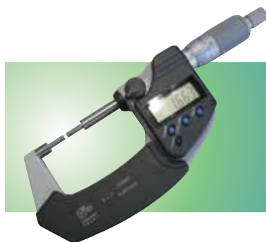
Figure 2a. Spline type micrometre with reduced measuring face
