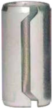
**Dowel Bushings** are used to locate components in conjunction with bolts which pass through the inside of the Dowel after it has been installed. Separate holes for locating pins are eliminated. The hardened Dowels also absorb shear loads, isolating the bolts from these forces.
