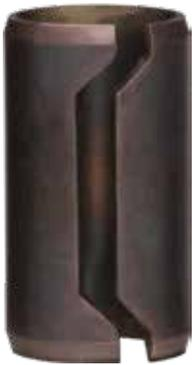
**Spring Dowels** are used to accurately locate components with respect to each other. They are formed around arbors to assure roundness. It is recommended that one half the hole tolerance be used for the fixed location of the Dowel and one half for the hole in the mating part.
