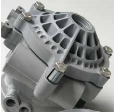
In applications where the mating component is also plastic, a Compression Limiter is necessary to avoid the creep or stress relaxation in the mating component from reducing the frictional load in the threaded joint.
